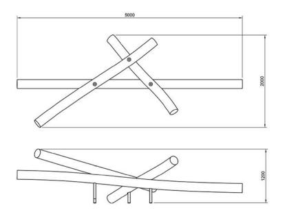
Ideal for a natural play setting, the Robinia 3 log stack is a great playground addition. Made from our highly durable 200-250mm diameter robinia poles, the robinia 3 log stack is extremely robust whilst still offering an architecturally pleasing piece.
